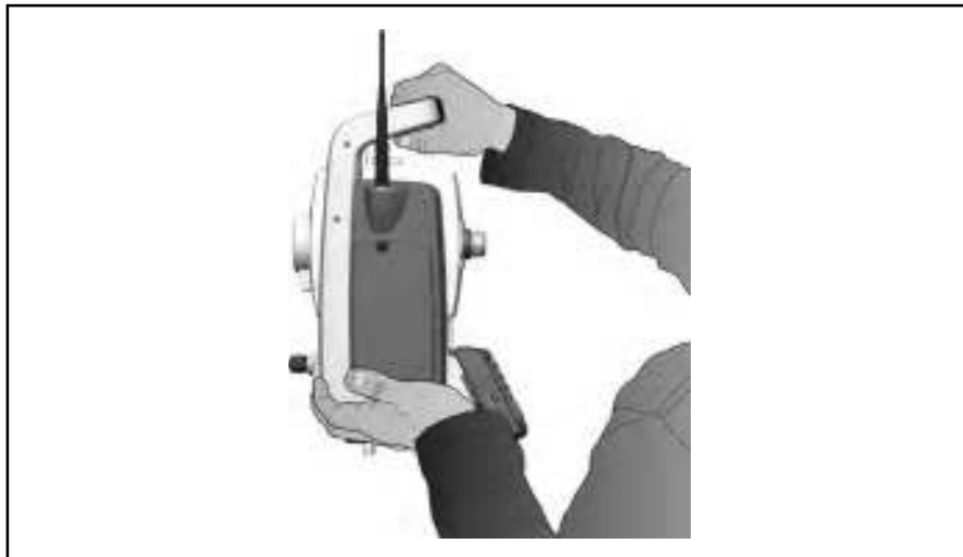
Figure 4.42 Correct way to lift the instrument
